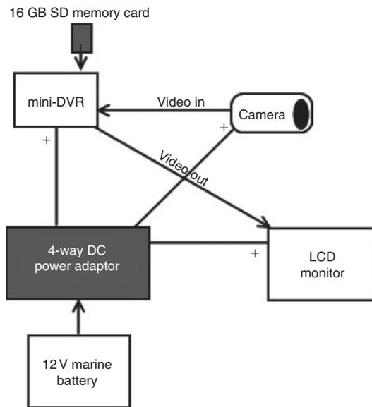
**Fig. 1.** Schematic design for using the underwater video camera (UVC) system to sample fish in dense submersed vegetation. A 12-V DC marine battery powers the system. Power adaptor connections to the digital video recorder (DVR), UVC, and video monitor are indicated with a + symbol. The 16 gigabyte memory card is used to store video recordings from the DVR. Video cables connect the camera to the DVR, and connect the DVR to the video monitor.
